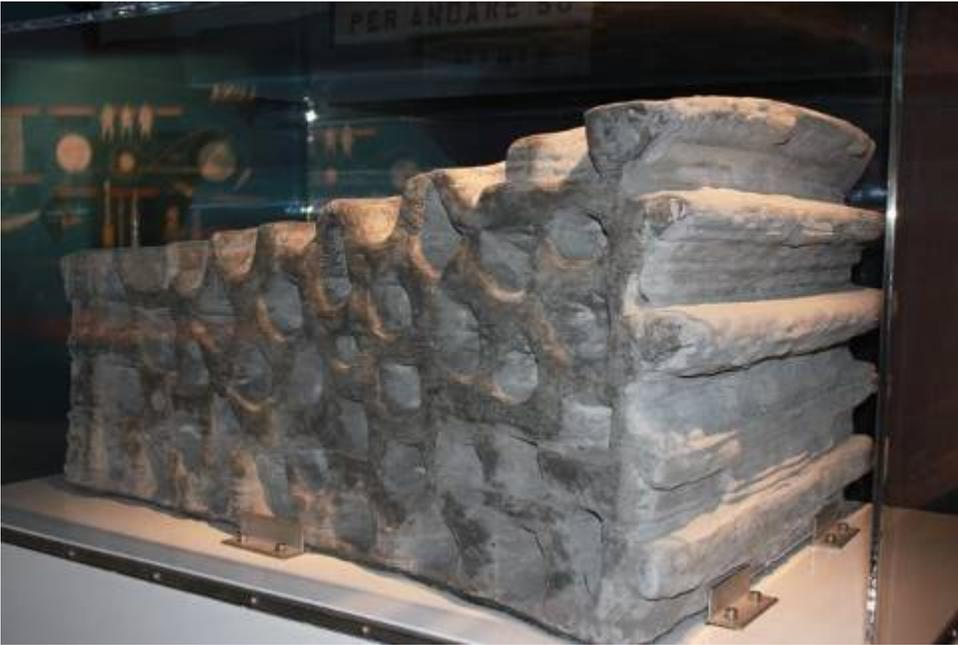
*This 1.5 tonne building block was produced as a demonstration of 3D printing techniques using lunar soil.
