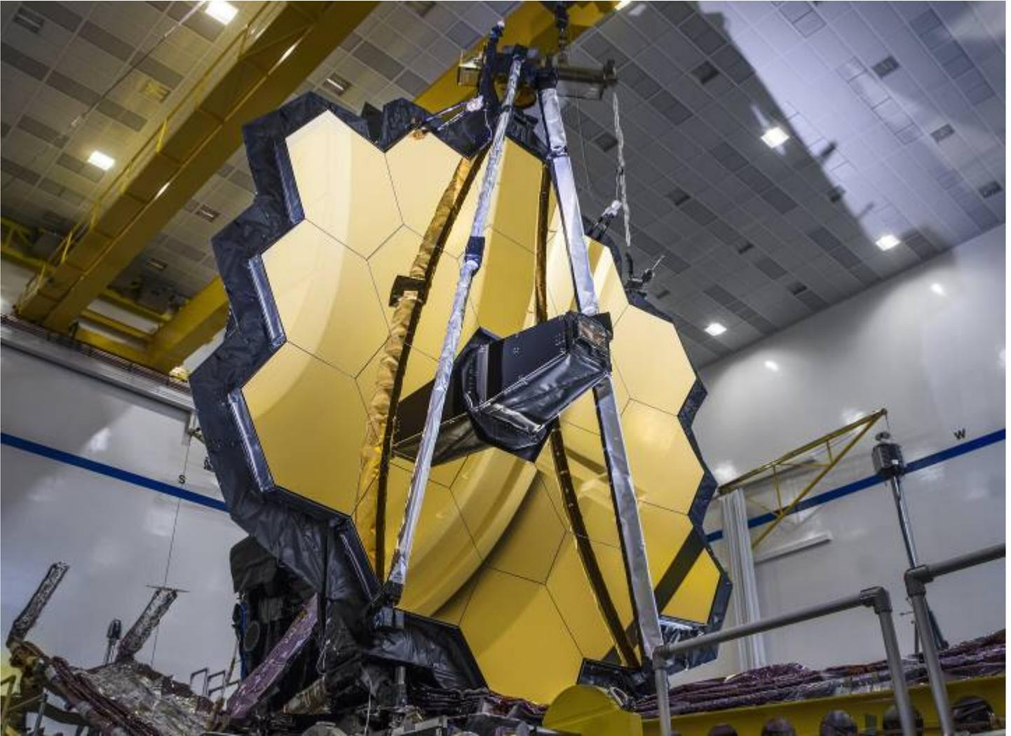
In a recent test, NASA's James Webb Space Telescope fully deployed its primary mirror into the same configuration it will have when in space.
