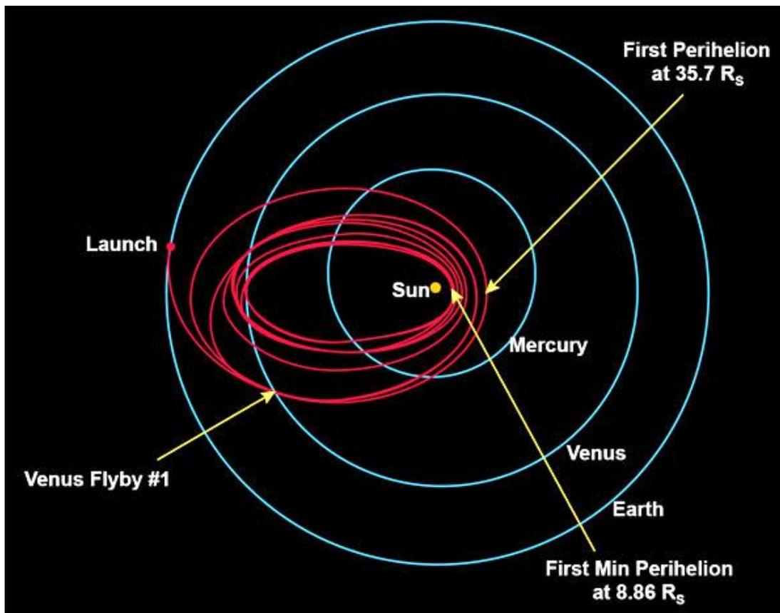
*Parker Solar Probe has completed two of the seven Venus flybys that will ultimately shrink its orbit around the Sun to within 9 times the solar radius.
