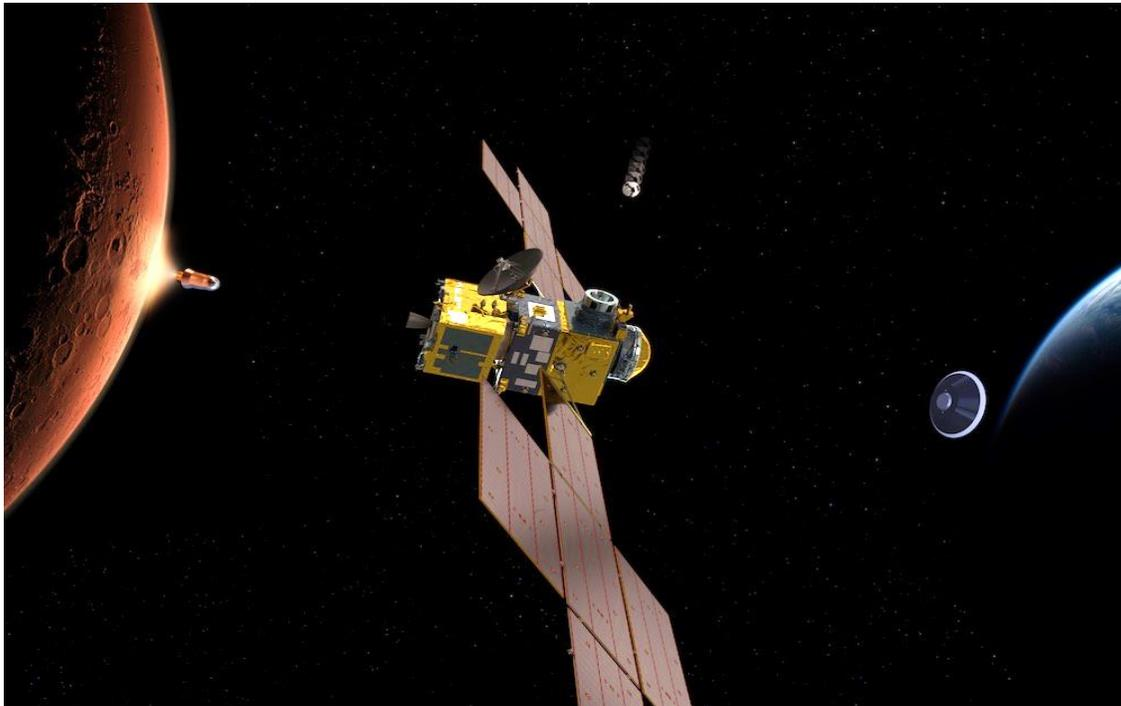
*Artist's concept of a Mars sample return mission, including a U.S.-built Mars Ascent Vehicle (left), a European-built Earth Return Orbiter (center), and a NASA-provided Earth Entry Vehicle (right). Credit: ESA/ATG medialab*
