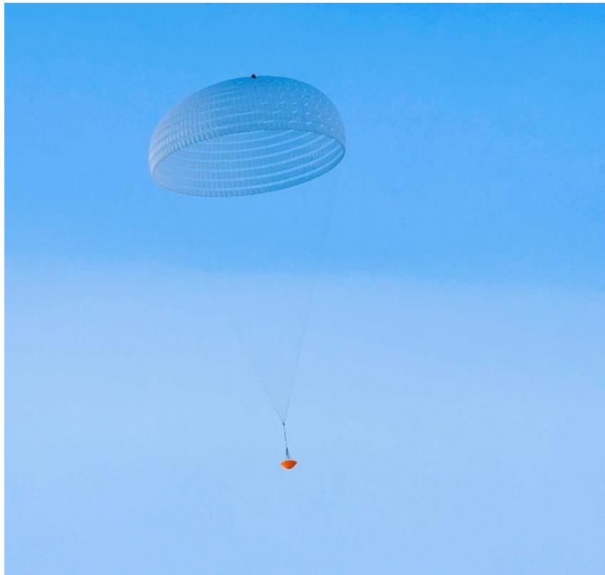
*The deployment of the large 35 m-wide parachute of the upcoming ExoMars mission was tested previously in a low-altitude drop test earlier this month. The image captures the inflated ring-slot parachute with the drop test vehicle suspended underneath.*
