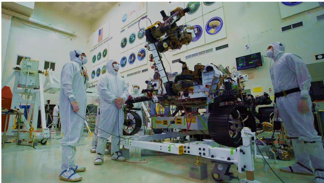
*In this image, taken July 19, 2019, in the clean room of the Spacecraft Assembly Facility at JPL, the rover's 7-foot-long (2.1-meter-long) arm maneuvers its 88-pound (40-kilogram) sensor-laden turret as it moves from a deployed to a stowed configuration. Credit: NASA/JPL-Caltech*
