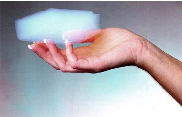
Silica aerogel is not what you might think it is. Rather than an actual gel, it’s a solid, rigid, dry material. It’s created by extracting the liquid from a gel with a process called [supercritical drying](#), the same process used make decaffeinated coffee.
