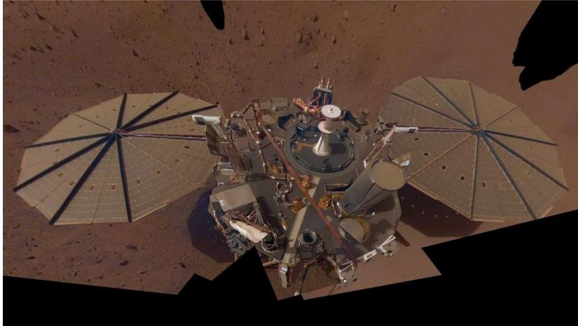
*This is NASA InSight's second full selfie on Mars. Since taking its first selfie, the lander has removed its heat probe and seismometer from its deck, placing them on the Martian surface; a thin coating of dust now covers the spacecraft as well.*
