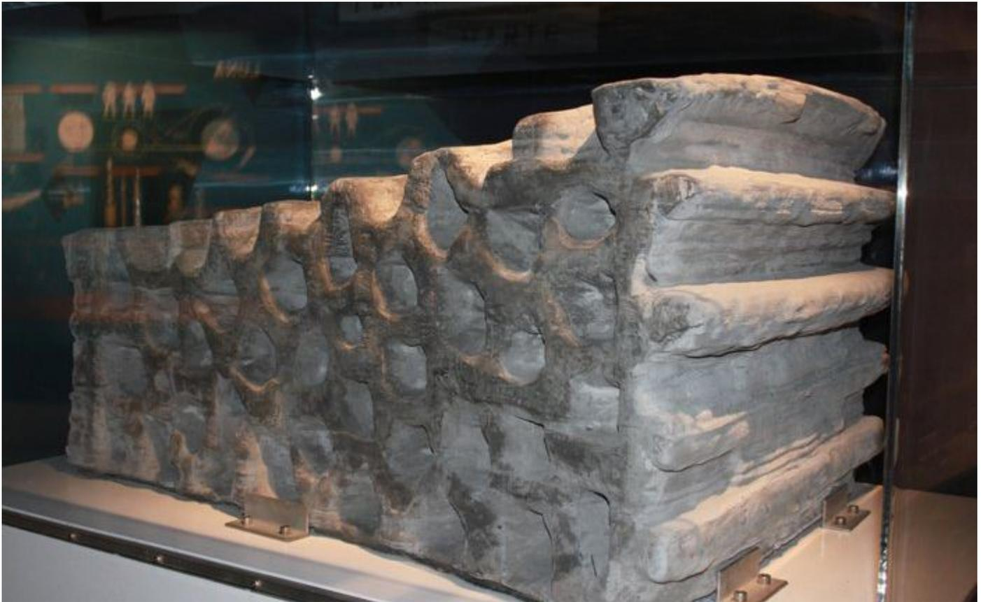
*This 1.5 tonne building block was produced as a demonstration of 3D printing techniques using lunar soil. The design is based on a hollow closed-cell structure – reminiscent of bird bones – to give a good combination of strength and weight. Credit: ESA*
