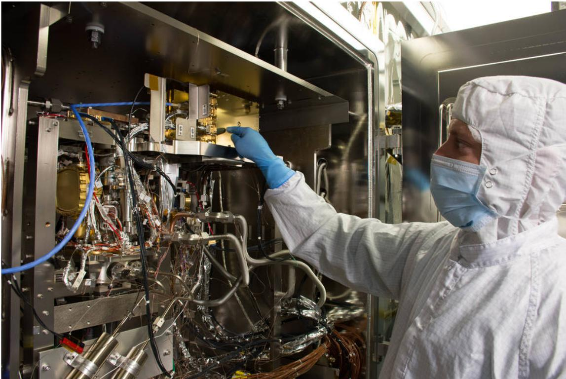
An international team of scientists has created a tiny chemistry lab for a rover that will drill beneath the Martian surface looking for signs of past or present life. The toaster oven-sized lab, called the Mars Organic Molecule Analyzer or MOMA, is a key instrument on the [ExoMars Rover](#), a joint mission between the European Space Agency and the Russian space agency Roscosmos, with a significant contribution to MOMA from NASA. It will be launched toward the Red Planet in July 2020.
