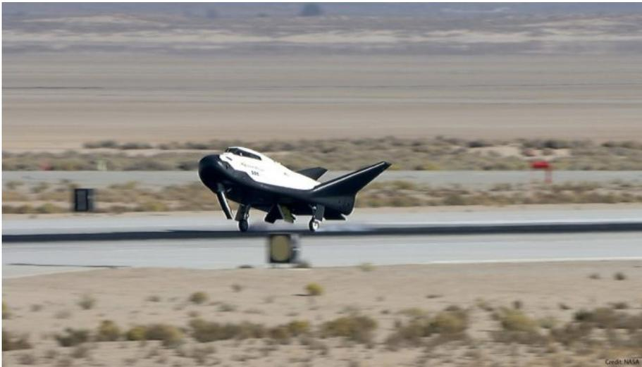
An atmospheric test article of Sierra Nevada Corp.'s Dream Chaser spaceship made a successful runway landing Saturday at Edwards Air Force Base in California after a glide test flight performed to verify the craft's handling qualities and guidance systems before future resupply missions to the International Space Station.
