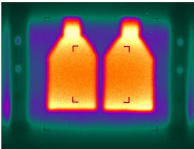
*Plastic bottles which were shot with ions from the Galactic Cosmic Ray simulator beam at the NASA Space Radiation Laboratory. Credits: U.S. DOE, Brookhaven National Laboratory, NA*
