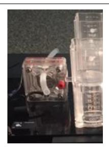
Put alcohol on a piece of paper towel and use it to wipe the ends of the tubes.
