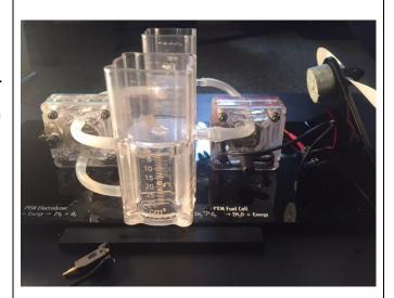
Remove the black caps briefly to allow hydrogen and oxygen to flow through the fuel cell.
