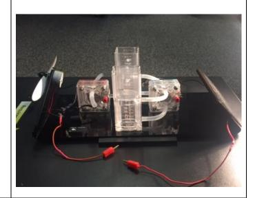
Make sure the black caps are **covering** the vents on the fuel cell. They should be **ON**.
