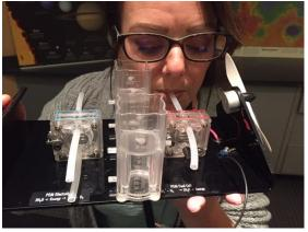
Connect both the red and black cables from the solar cell to the electrolizer.
