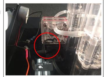
Use the pipette to adjust the water level as needed; making sure the water level is below the tubes to the fuel cell.
