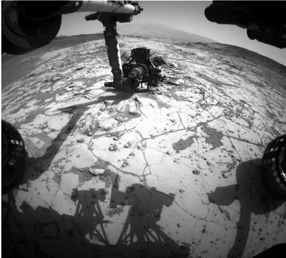
*This view from the wide-angle Hazard Avoidance Camera (Hazcam) on the front of NASA's Curiosity Mars Rover shows the rover's drill in position for a mini-drill test on Jan. 13, 2015. Credit: NASA/JPL-Caltech*
